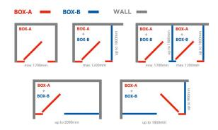
For guidance on standard toilet cubicle sizes referencing Building Regulations Part M and the Equality Act 2010 visit - www.washroomcubicles.co.uk/toilet-cubicle-sizes/
