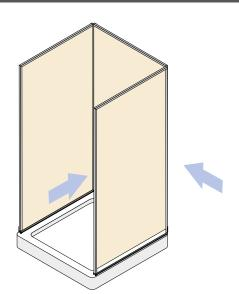
Attach a third **Seal channel** to the shower tray in the initial stages. (Step 3 & 4)
