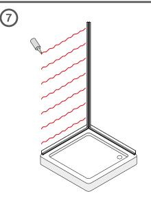
Apply thick beads of **adhesive** in multiple lines onto the wall. Ensure top, middle and bottom areas are covered. Use a full tube of **adhesive**.
