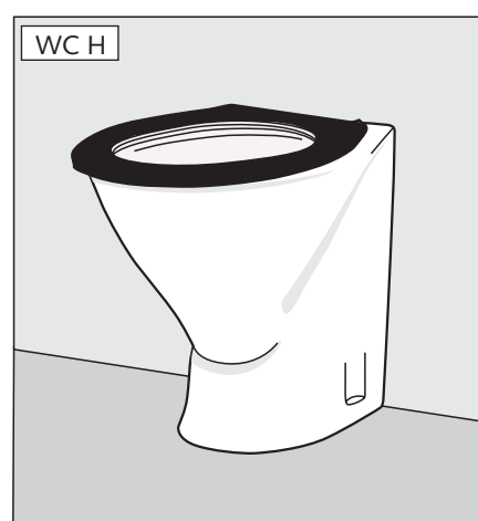
Figure 10 WC for ambulant and semi-ambulant users
